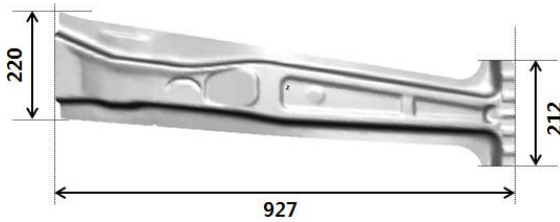
Fig. 1 Shape and dimension of the center pillar member
