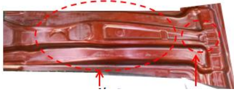
Fig. 7 Die spotting status after the surface treatment
