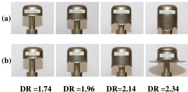
Fig. 5 Photographs of drawn specimen for various DRs; (a) with and (b) without ultrasonic vibration
