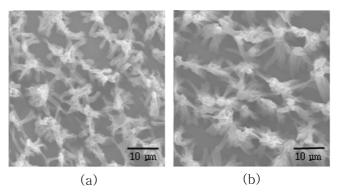
Figure 2. SEM images of tubules prepared with different numbers of potential cycling. (a) 5 cycles; (b) 15 cycles. The template membrane was removed.
