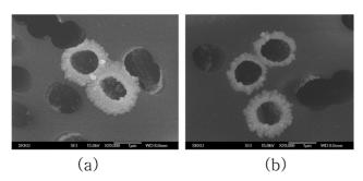
**Figure 7.** SEM images ( $\times$ 20000) of the microtubule electrode array after electrochemical deposition of HAuCl<sub>4</sub> solution by chrono-amperometry (duration time=10 sec (a); 100 sec (b)).
