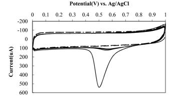
Figure 4. Cyclic voltammograms of microtubule array electrode in  $0.5 \text{ M H}_2\text{SO}_4$  with (line) and without (dashed) 1 mM HAuCl<sub>4</sub>. Scan rate = 50 mVs<sup>-1</sup>.
