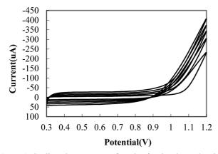
**Figure 1.** Cyclic voltammogram of EDOT for the electrochemical polymerization in the 1.2  $\mu$ m pores of the template membrane. The solution is 0.1 M EDOT in acetonitrile containing 0.1 M LiClO<sub>4</sub>. Potential scan from 0.3 to 1.2 V was performed 5 cycles *vs.* Ag/AgCl (Sat'd KCl). Scan rate is 50 mV/s.
