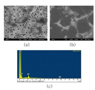
**Figure 3.** SEM images (a, b); EDAX data (c) of PC membrane  $(1.2 \ \mu m \text{ pore size})$  sputtered with gold. (a), (c) from gold-sputtered surface and (b) from the opposite side.
