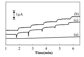
**Figure 8.** Comparison of responses to  $H_2O_2$  between naive (a); gold-treated (b,c) tubule electrode. (b) is the electrode from gold-sputtered membrane; (c) is the electrochemically gold-deposited electrode.  $H_2O_2$  was increased gradually from 0 to 0.5 mM by 0.1 mM step. (*E*=0.7 V vs. Ag/AgCl, counter=Pt plate).
