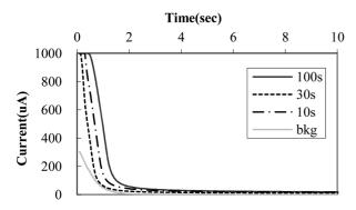
**Figure 6.** Chronoamperograms of microtubule array electrode for gold deposition. Duration time = 10, 30, 100 sec in 1 mM HAuCl<sub>4</sub>/ 0.5 M H<sub>2</sub>SO<sub>4</sub> and 100 sec in 0.5 M H<sub>2</sub>SO<sub>4</sub> (background). Potential step = 0.9 V to 0.2 V vs. Ag/AgCl, counter = Pt plate.
