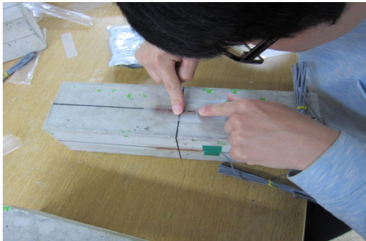
(a) Installation of concrete strain gauges
