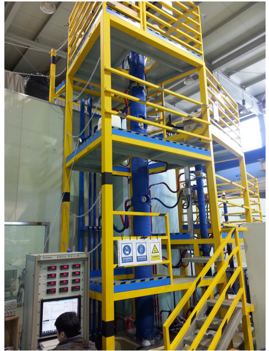
Fig. 4 Underwater acoustic performance measurement system(pulse tube)
