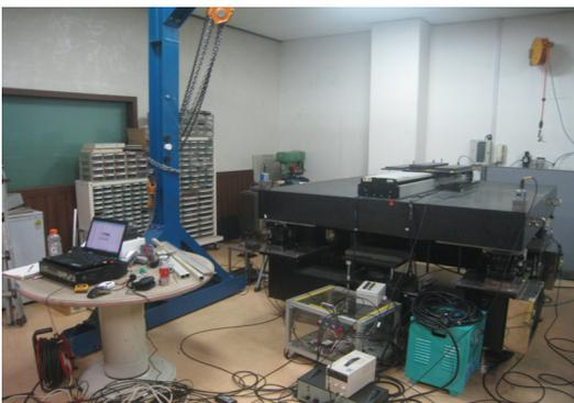
Fig. 3 Modal testing of the isolation table
