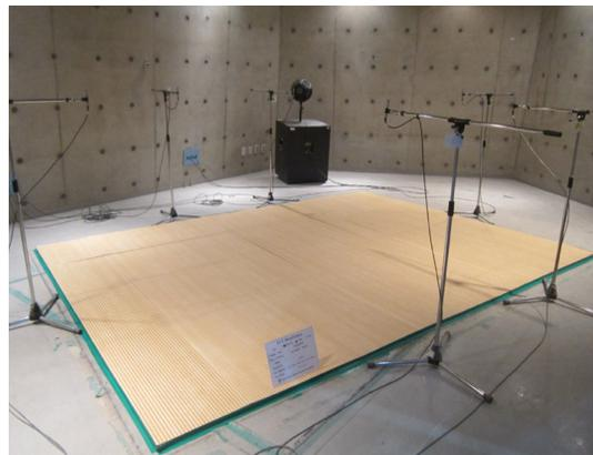
**Fig. 2.** Sound absorbing test of carbonized board and prototype of complex board.
