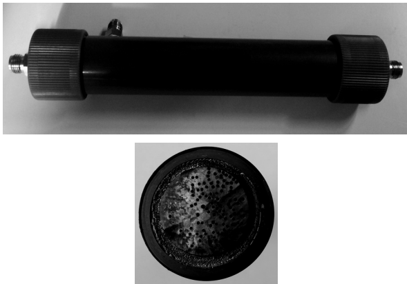
Fig. 1. Hollow fiber membrane module and housing prepared at Airrane Co. Ltd..
