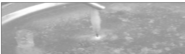
Fig. 4. Spark discharge of needle end point in solution.
