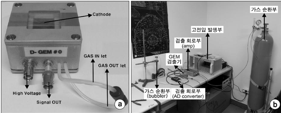
Fig. 1. (a) GEM detector, (b) GEM detector system.
