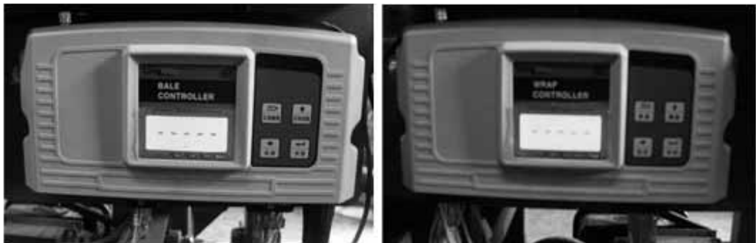
Fig. 12. Controllers of baling and wrapping.
