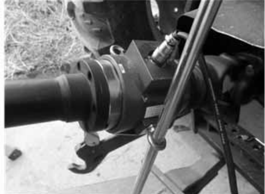
Fig. 17. Measuring the absorbed power in baling and wrapping process.
