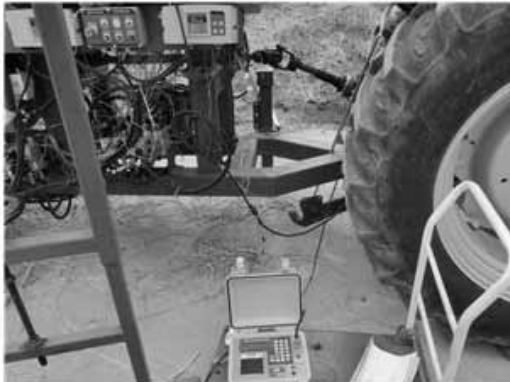
Fig. 17. Measuring the absorbed power in baling and wrapping process.
