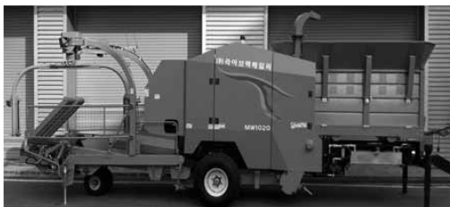
Fig. 7. Bale-wrapping combined machine.
