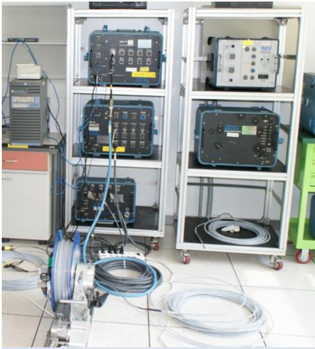
Fig. 6 Layout of the eddy current testing equipments for inspection
