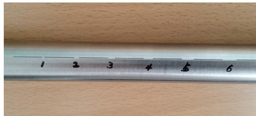
Fig. 5 EDM notch specimen containing collinear cracks
