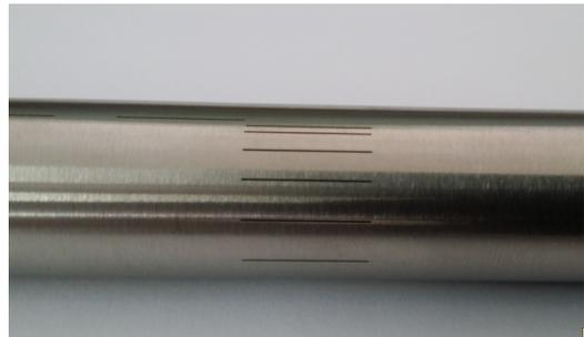
Fig. 4 EDM notch specimen containing parallel cracks
