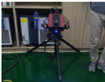
(b) 3D scanning equipment
