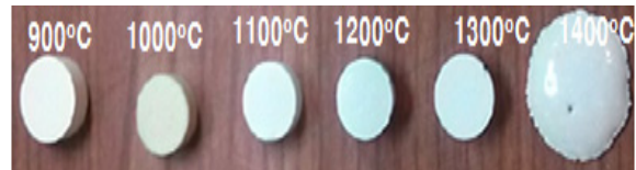
Fig. 4. Optical photographs of MASZ2 samples after heat treatment at various temperatures.
