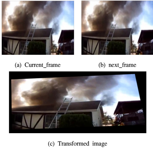
Fig. 8. Transforming next frame according to current_frame of the stabilization algorithm is shown in [fig. 9].
