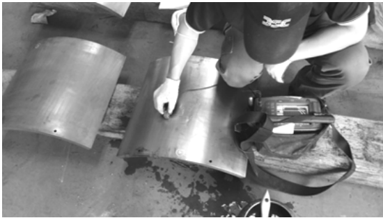
Fig. 9 Ultrasonic test of specimens after full-scale HIC test
