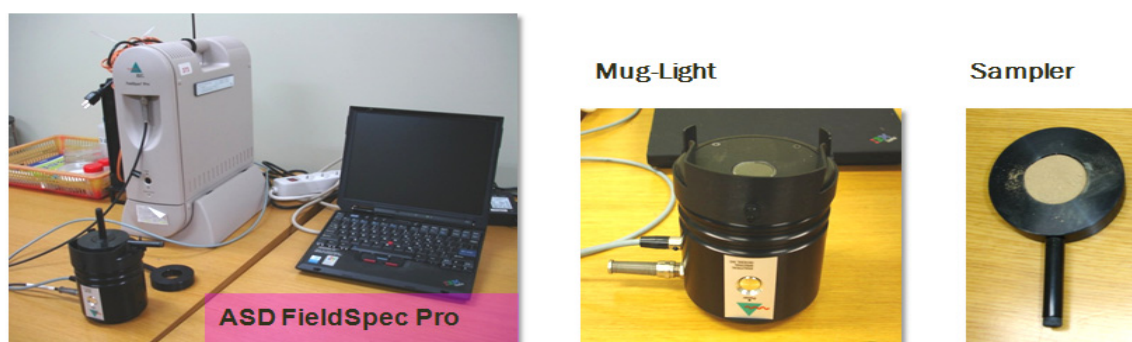
Fig. 1. Spectral reflectance measurement from 350 nm to 2,500 nm using ASD FieldSpec Pro (Applied Spectral Devices, Boulder, CO).
