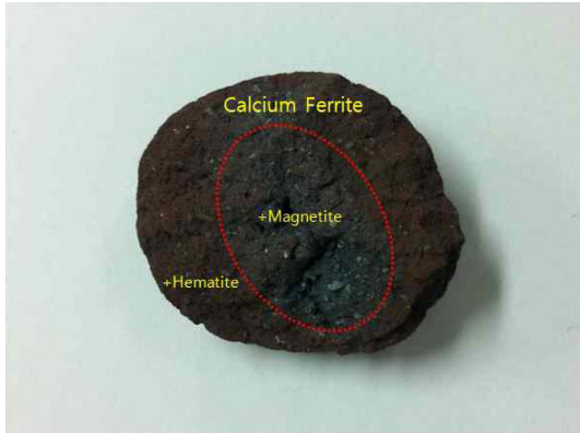
Fig. 6. Photograph of cross section of calcium ferrite specimen(NO. 3) at 1100°C.
