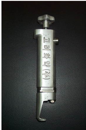
Fig. 6. Impact blaster of non electric detonator.
