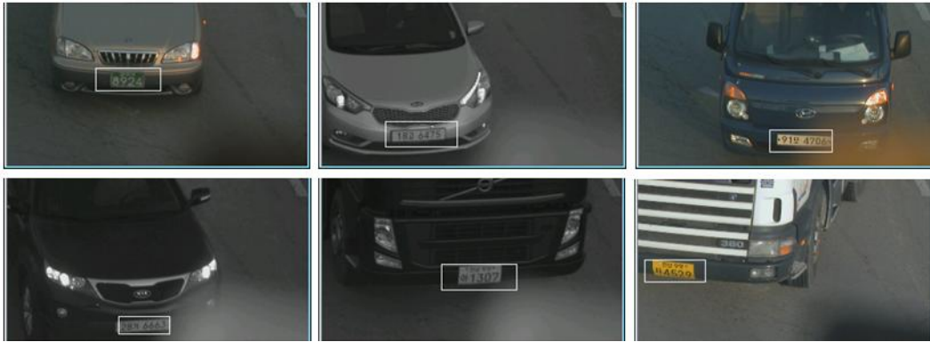
Fig. 19. Examples of successfully detecting license plates from cars under different conditions using the proposed method
