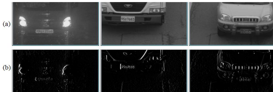
Fig. 12. Examples of image pre-processing results: (a) results after using the Gaussian filter (b) results after using the Sobel vertical operator
