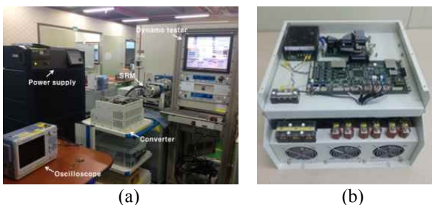
Fig. 17. Experimental set up with the first prototype of permanent-magnet-assisted SRM: (a) testing installation; (b) converter drive
