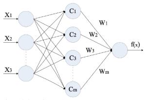
Figure 1. A Typical Three-Layer RBF Neural Network
