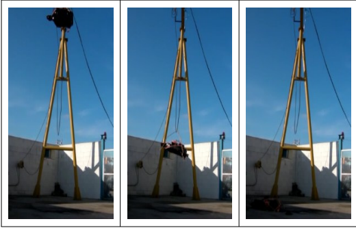
Fig. 7 The experimental apparatus for drop test
