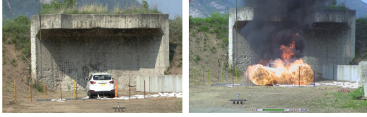
Fig. 12 Fire status of the HFCV
