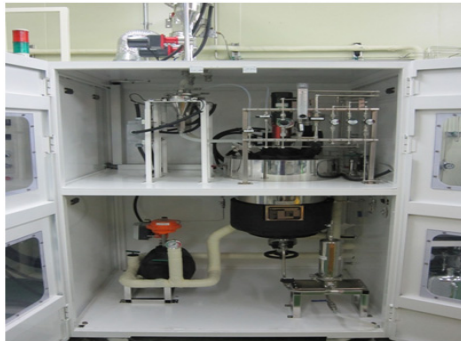
Fig. 1 Schematic diagram (a) and system (b) Ammonia borane synthesis process
