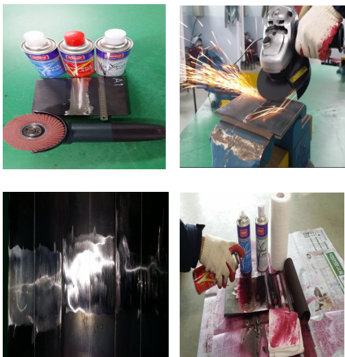
[Fig. 4] Penetrant inspection test equipment and surface treatment
