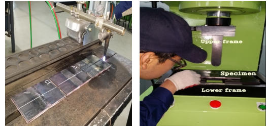
[Fig. 5] Specimen processing, cutting and bending test experimental equipment
