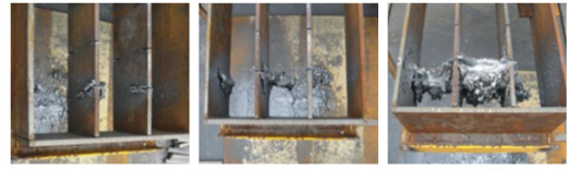
[Fig. 4] Cutting support after repeated cutting
