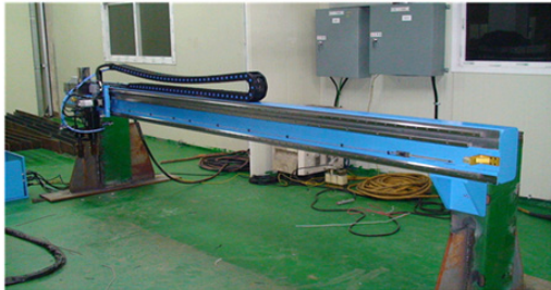
[Fig. 9] Dross cleaning system
