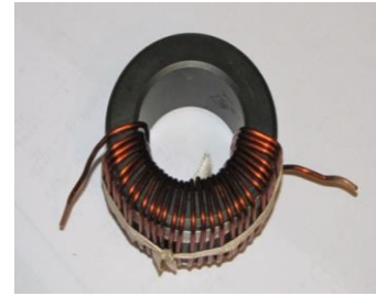
Fig. 12. Inductor b: toroidal inductor with a ferrite core of type OR66x38_30H produced SAMWAH Company
