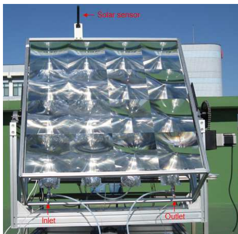
Fig. 9 Validation of the heating system using a CPV grid
