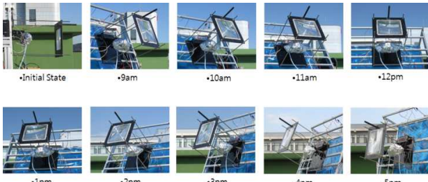
Fig. 4(a) Transient motion of the heating system as a function of time
