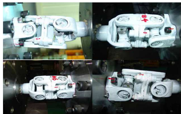
Fig. 6 Failure of the propeller shaft test
