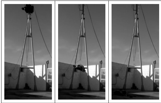
Fig. 5. The experimental apparatus for drop test
