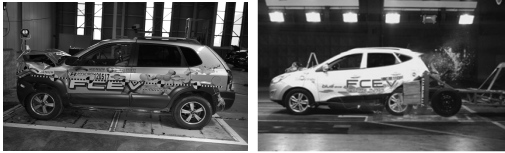
Fig. 1 The test vehicle of frontal and rear impact test
