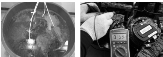
Fig. 6 The experimental apparatus for immersion test
