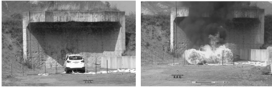
Fig. 8. Fire status of the HFCV
