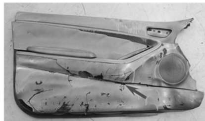
Fig. 4 A case of map pocket end rupture
