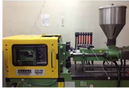
Fig. 6 Photo of injection molding machine (Arburg)
