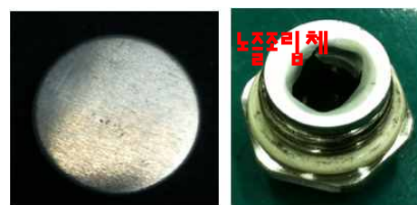
Fig. 3. Pre-Test-Post-Test of Rupture Disk
