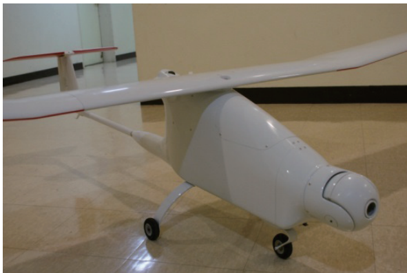
Fig. 7. HeXUS F-3 used for the flight test. It is equipped with a two-axis gimbal system
