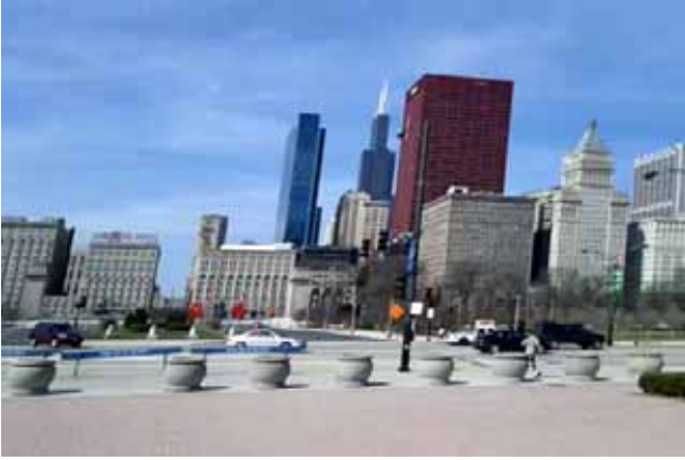
Fig. 2. Illustration of the rolling shutter effect. All the buildings appear slanted as the camera pans across the scene.
