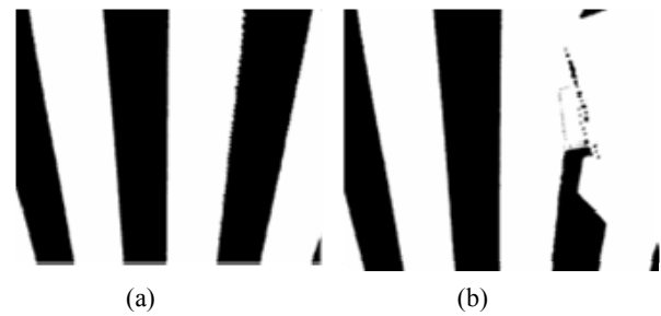
Fig. 9. Binarized image set of reference pattern reflection and pattern distortion (a) A binary image result for reference pattern projection, (b) A binary image for pattern projection onto our experimental objects.
