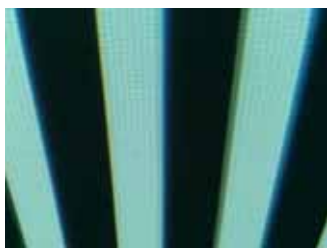
Fig. 7. Pattern projection image frame captured by a camera.
