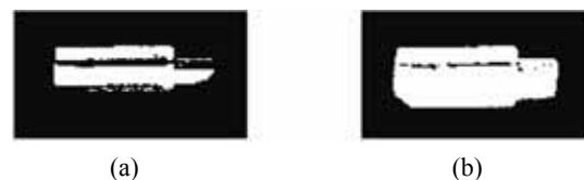
Fig. 2. Shadowed area of an object (a) Binary image with shadow removal, (b) The shadowed region is included as an object during image binarization.
