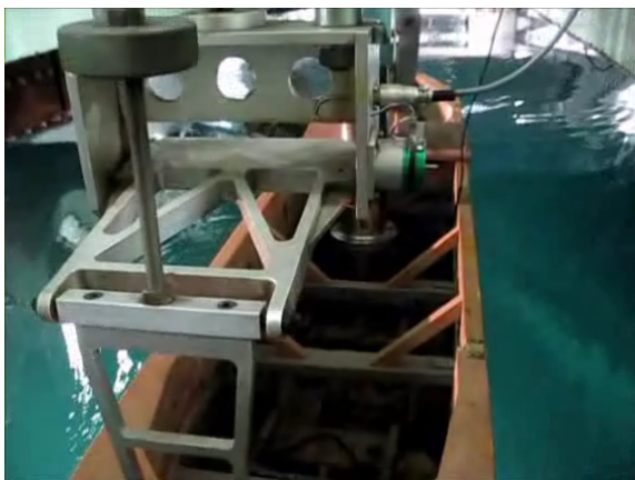
Fig.3 Test model equipped to towing carriage
