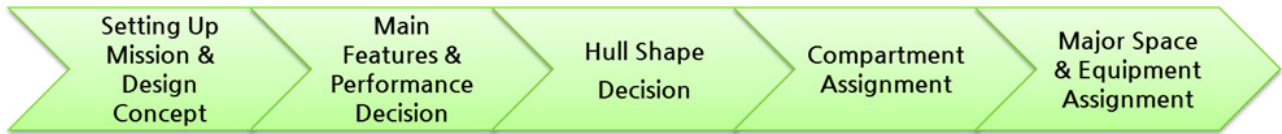
Fig. 1 General arrangement (GA) process of domestic naval ships
