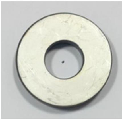
Fig. 4 Piezoelectric ring specimen
