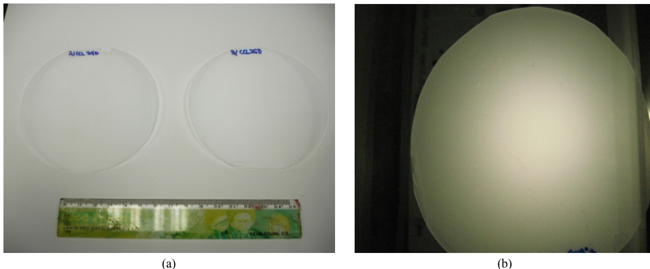
FIG. 2. (a) Appearance of UV-cured molding film (full scale of the ruler: 15 cm), and (b) transmitted light through the fabricated PC and PMMA sheets.
