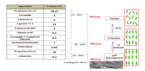
Fig. 3. Thermosensitive polymer non-hydrous skin analogous layer LC production flow mapping.
