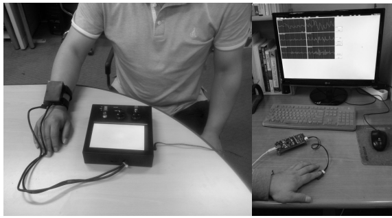
(a) a wrist-type prototype (b) finger-shaped prototype Fig. 4. The module of LED and camera that collect for biosignal
