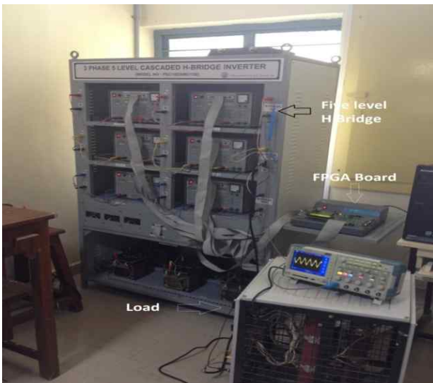
Fig. 9. Experimental setup of Five-level H-Bridge Inverter.
