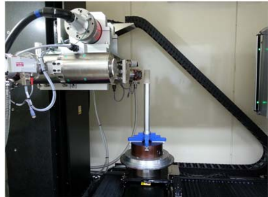
Fig. 2. View of X-ray CT scanning for Berea sandstone.
