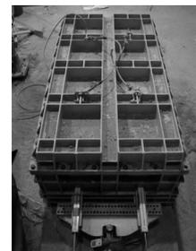
(c) Positioning an air bag to simulate normal pressure (d) Installing top cover of soil box and LVDT for displacement measurement
