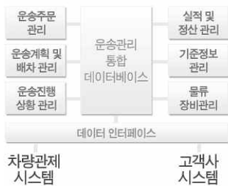
[Figure 2] TMS System Module
