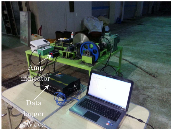
Figure 3. Data acquisition system for cutting power measurement.
