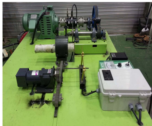
Figure 2. Cutting power measuring facility of fast growing trees.
