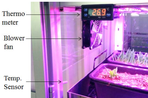
Fig. 4 Forced cooling system by air blower
