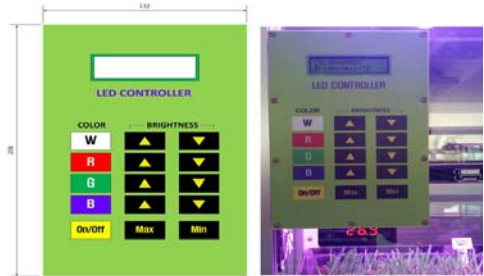
Fig. 3 LED controller for wavelength and illumination
