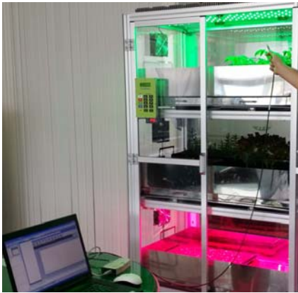
Fig. 9 Measuring wavelength of LED system
