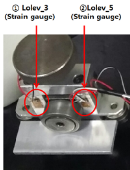
Fig. 5 Strain gages adhesion
