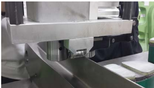
Fig. 15 Operation of Auto roll forming machine
