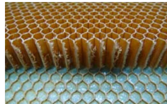
(b) Vertical wall(hogger cutter, 1,000mm/min)
